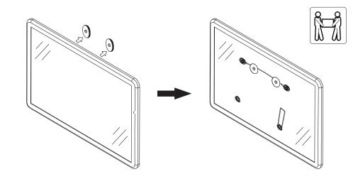
After the wall mount has been safely secured to the wall, Carefully lift your TV and hook wirerope into the wall plate rail. Make sure your TV is securely and correctly attached.
