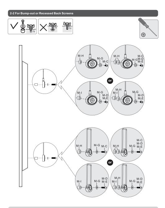
Note: Choose the appropriate screws, washers and spacers (if necessary) according to the type of screen. · Screw the supporting spacers onto the TV.
