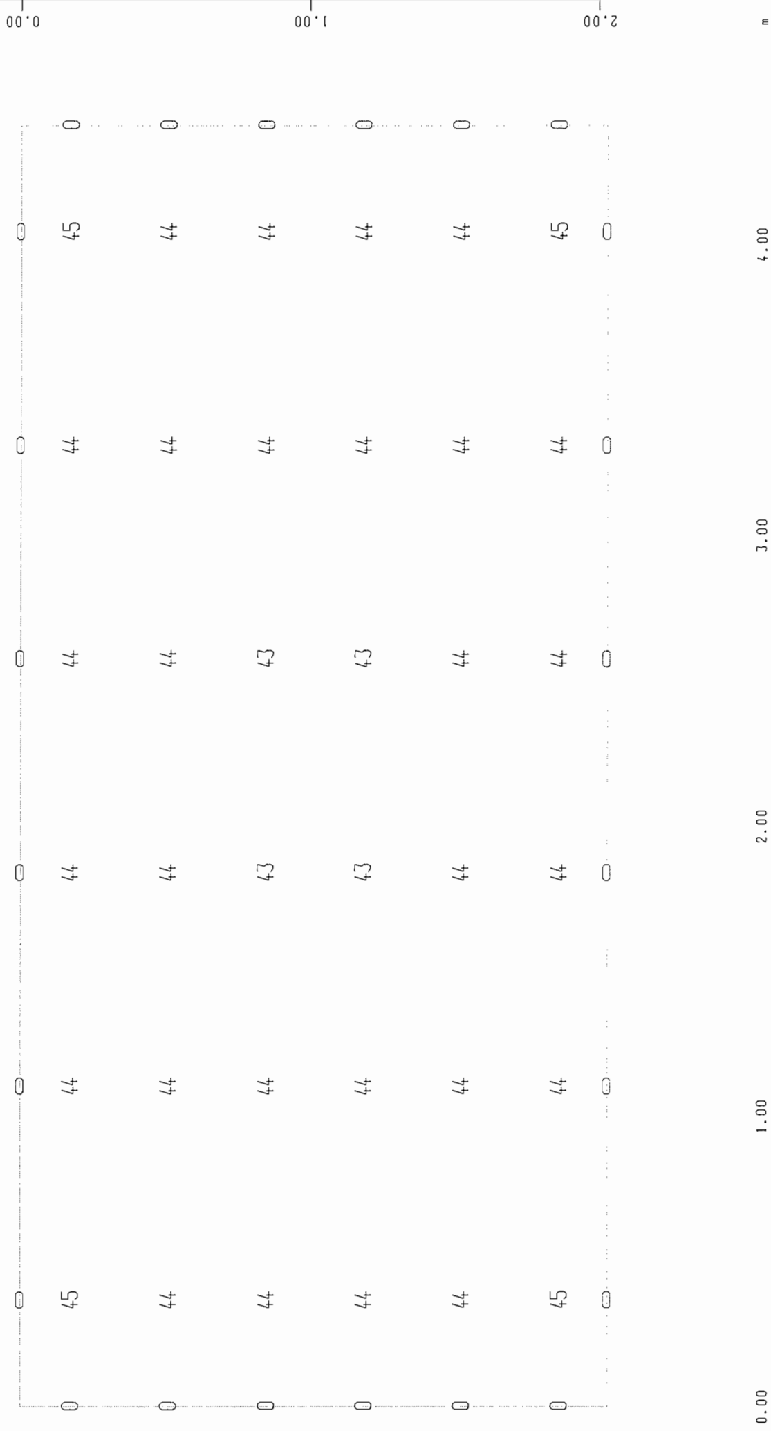
Bedding stresses in Elements in kN/m², Loadcase 1 (Min=-0.319) (Max=4.7)
