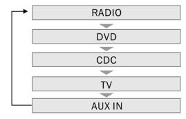
CDC/AUX IN can be skipped when no external devices are connected.
