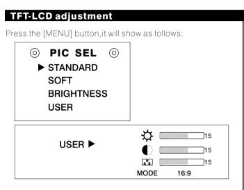
Press ▲ and ▼ to remote cursor up and down, and press ◀ or ▶ to adjust.
