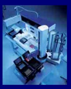
QIAGEN's BioRobot<sup>®</sup> instrumation platform + Zymark's 96/384-well pipetting solutions + Zymarks Twister<sup>TM</sup> robotic arm system
