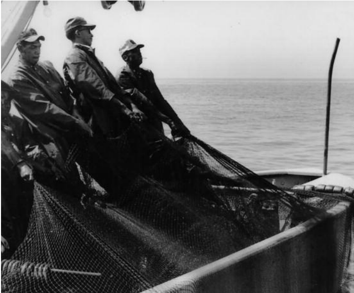
Crew hauling in the purse seine by power block
