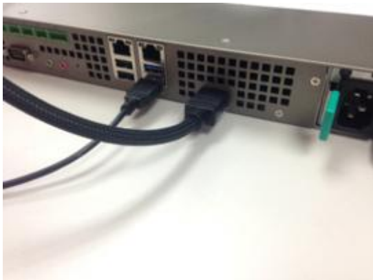
Connect the Keyboard and monitor to NVR
