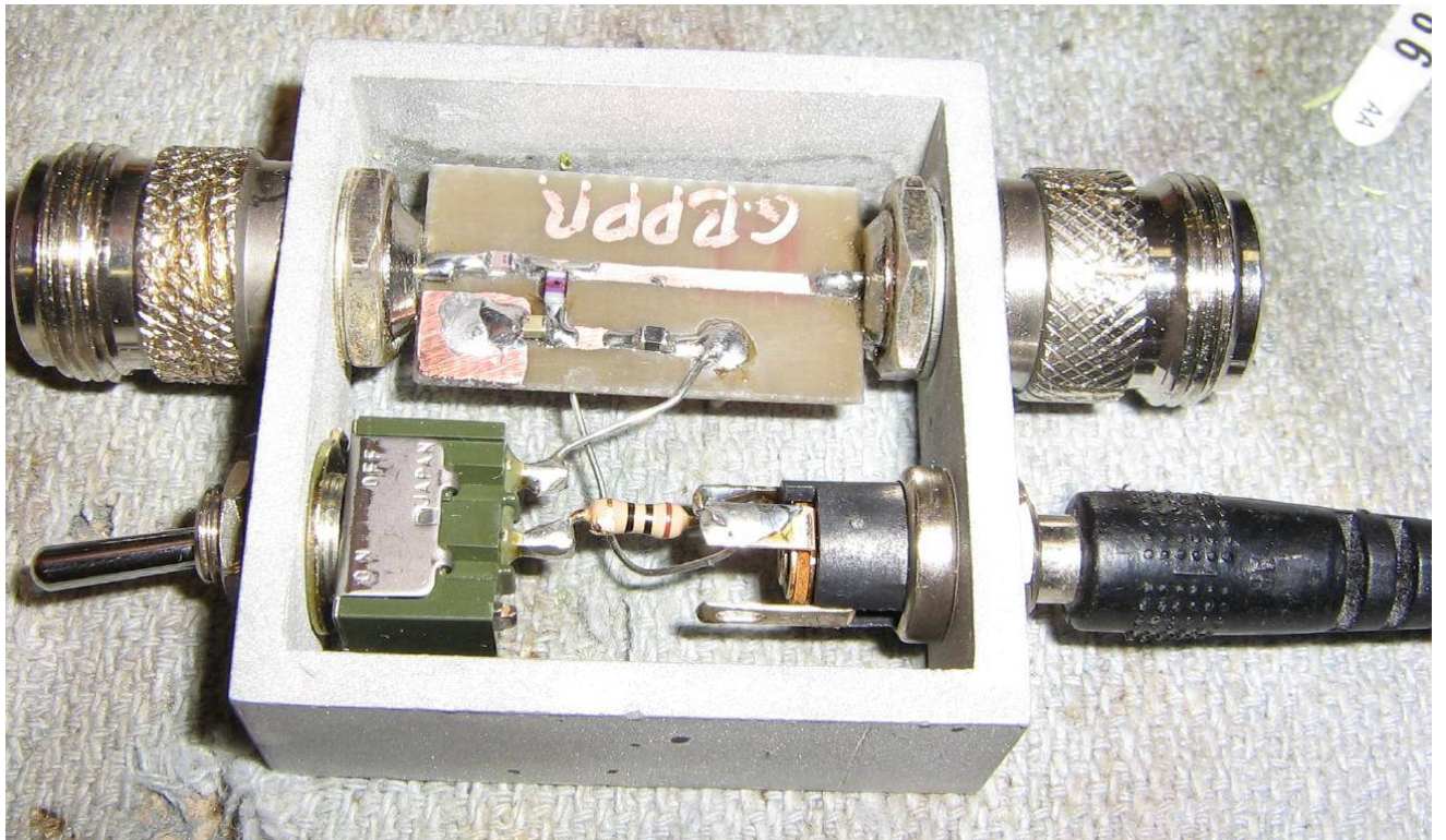
Overall view of the finished bias-tee. There is not much to it. The DC voltage comes in via a 12 volt wall-wart power supply and is controlled via a SPST select switch. A 10 ohm resistor acts as a current limit and fuse. The radio connects to the left-side N connector. The switch circuit and DC-inject signal connect to the right-side N connector.
