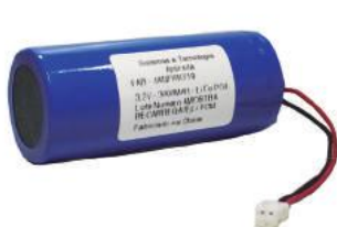
3,2V 3000mAh • LiFePO 4 • Conector A58 • c/ PCM • 26x65mm 036084
