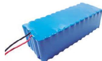
48,1V 13S5P • 236x92x68mm • c/ placa PCM MOD 5 036198 - 1500mAh
