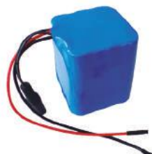
11,1V 3S3P • 56x56x68mm • c/ placa PCM MOD 3 036183 - 6600mAh 036184 - 7800mAh
