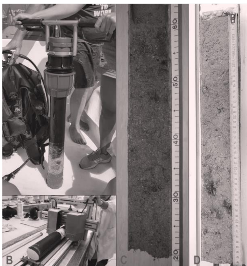
Fig. 1: A) Hand-corer used to collect the sediment cores; B) Instrument used for core sectioning; C) sectioned core (from 2018 sampling); D) sectioned core (from 2019 sampling).
