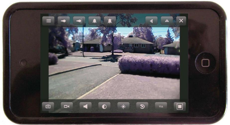
Figure 4: IP camera remote video and audio feed via proprietary iOS software running on iPod (my first, cheap IP camera's full-time IR filter in daylight turns green colours to violet).
