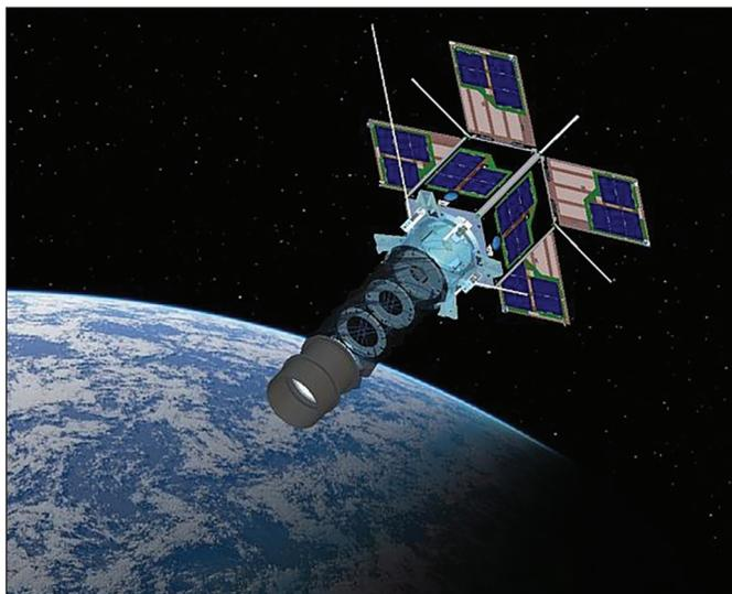
PRISM obtains its 10 metre resolution images using a colour CMOS area imager (1280 x 1024 pixel image size). This relatively high resolution from a small satellite was achieved by deploying the lens on an extendable boom mechanism that was successfully deployed on February 27, 2009.
