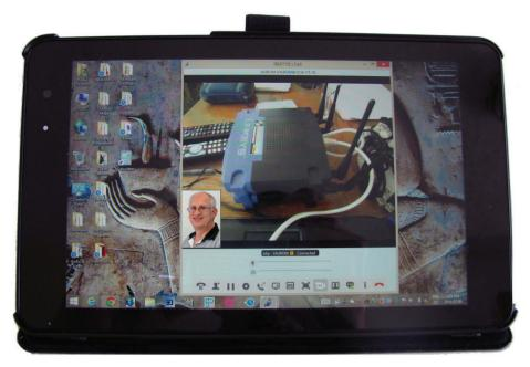
Figure 8: Jitsi on my Windows tablet connected the BBHN Mesh via Wi-Fi AP.
