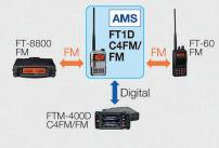
This is made possible in System Fusion by the Auto Mode Select (AMS) function. FM DR-1X FM Digital Digital AMS transmit
