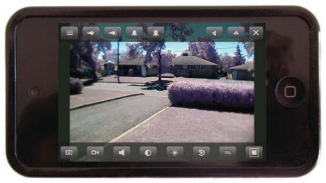
Figure 4: IP camera remote video and audio feed via proprietary iOS software running on iPod (my first, cheap IP camera's fulll-time IR filter in daylight turns green colours to violet).
