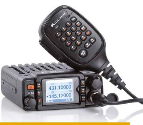
operating in VHF and UHF bands; it's a compact equipment with a modern and stylish design Amongst the many features supplied with CT2000, we point out the considerable output power of 25W (adjustable), which can be compared to the one of professional transceivers. CT2000 is a small-size radio, equipped with a powerful 3W speaker that guarantees an excellent audio quality and with a wide graphic multicolor display that allows easy observation of all settings and parameters.
