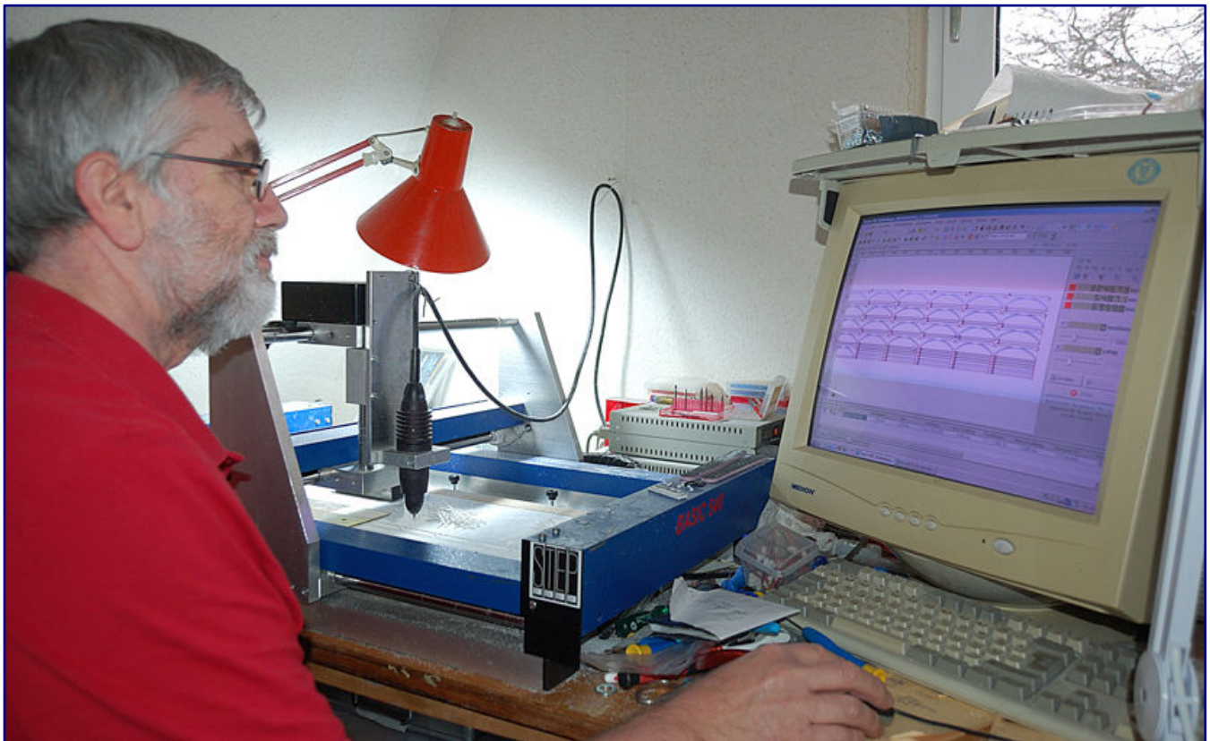
After the model research, the drawing on the computer follows, before the milling machine (middle) can start working out the structures on polystyrene plates. Photo: Rainer Tielke
