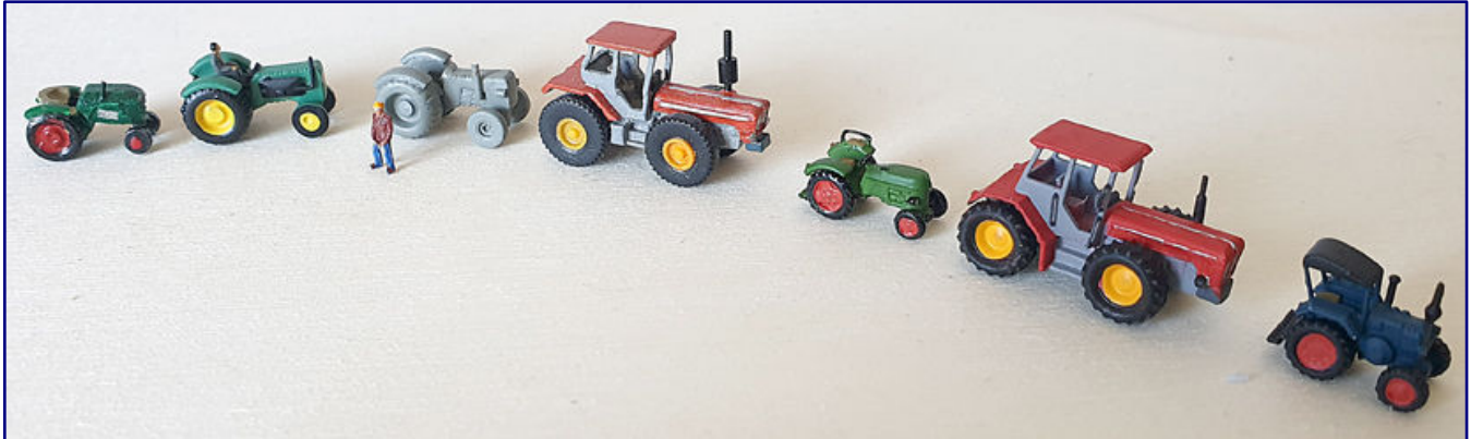
Chronology of an evolution (left to right): hand carved tractor from the early days, a MAN with laser cut chassis, a prototype with laser cut chassis, a FDM based Schlüter-tractor (consisting of 10 parts), and three SLA printed models: a Deutz D25, a Schlüter TVL2000 and a Lanz. Photo: Michael Hering
