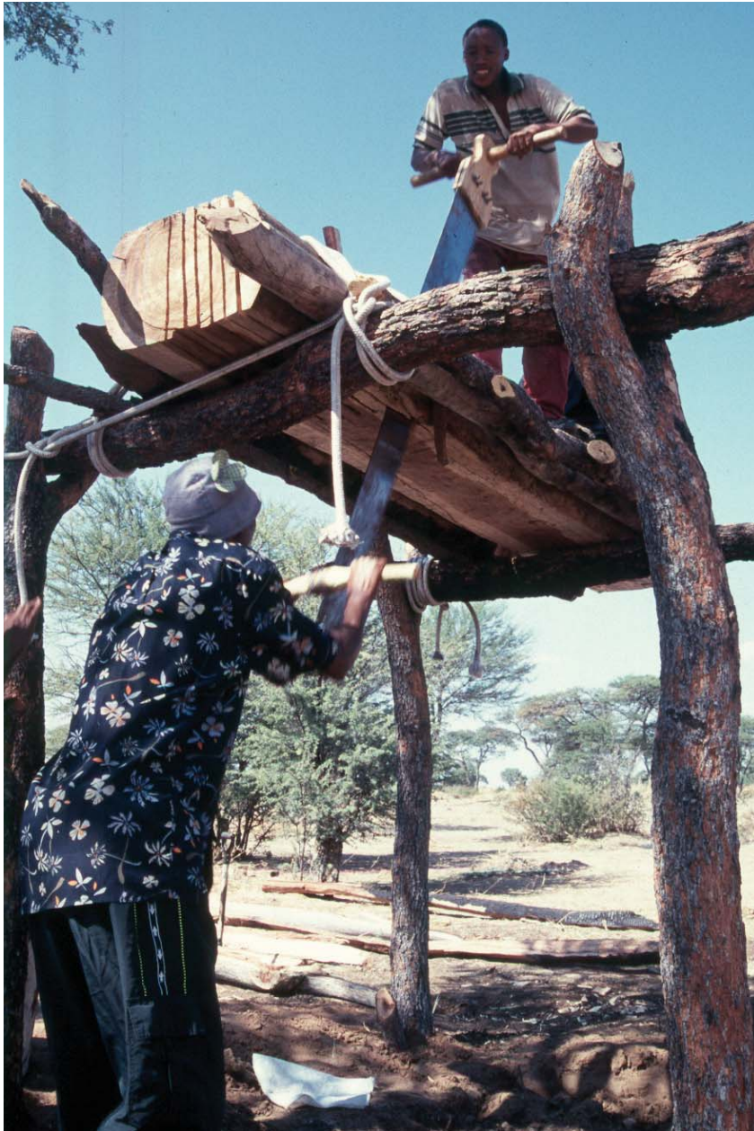
A pit-saw in operation, in this case mounted on stilts instead of in a pit in the ground. Cutting timber in this way is not easy, especially if straight planks with an even thickness are to be produced.
