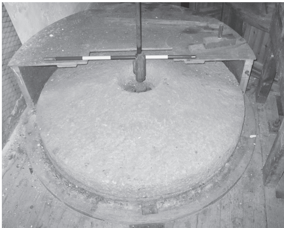
Fig. 14: Granite millstone from the Mourne Mountains in the restored watermill at Annalong, Co. Down. Photo: N. Colfer.
