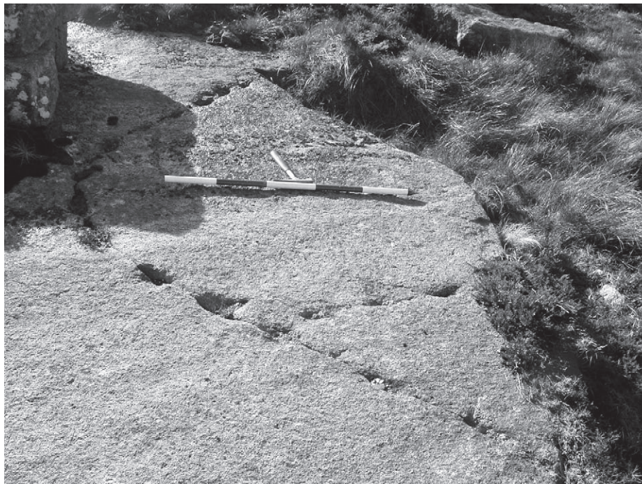
Fig. 8: Use of circular lines of vertical wedge pits or to produce semi-circular slab of stone. The intended millstone shape is also visible within the larger circle. Photo: N. Colfer.
