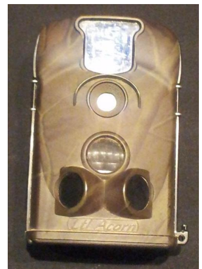
This “LTL Acom” scouting camera is a regularly used device to monitor animals in captivity and in the wild. It takes videos or motion sensed photos. Photo J.Marten
