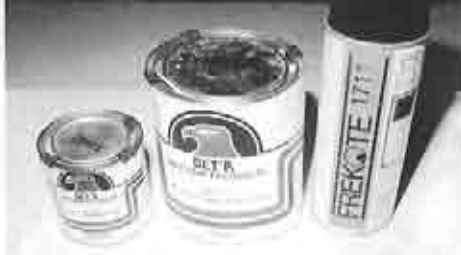
Figure 1 Release Agent Frekote 1711 & Bet'r Surface Coat BE-115.
