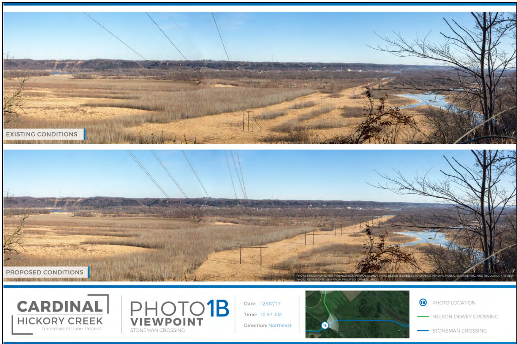
Figure 3.11-24. Visual simulation from viewpoint 1 showing Alternative 2 in the Refuge to the Mississippi River Crossing at the Stoneman Substation.
