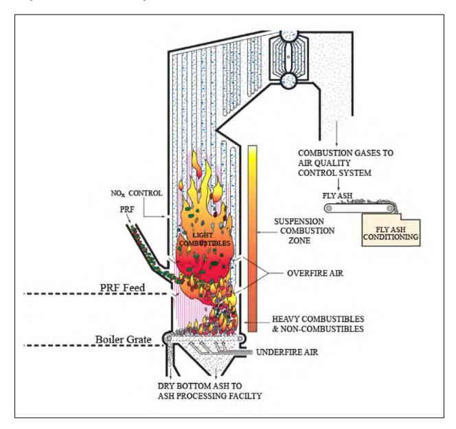
Figure 2-4. Processed Refuse Fuel Combustion in Spreader-Stoker Boiler
