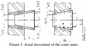
If the interior cone is executed at the superior limit of the  $D_{max}$  diameter, and the exterior cone at the inferior  $d_{min}$  diameter, there is an axial movement, AL.
