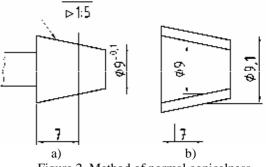
Figure 2. Method of normal conicalness a) the drawing; b) the tolerance field
