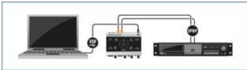
KOMPLETE AUDIO 6 connected to a DAT tape deck.
