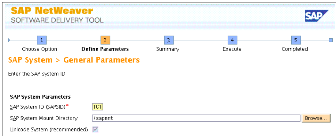
Figure E-3 SAPinst ASCS installation screen capture 3: SAP system ID and /sapmnt directory
