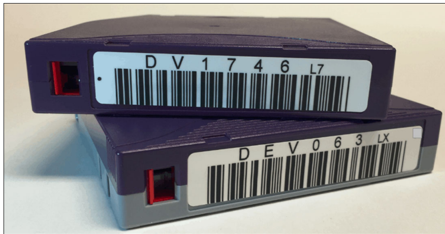
Figure 2-12 LTO-7 data cartridge (purple) and WORM cartridge (purple with platinum bottom)
