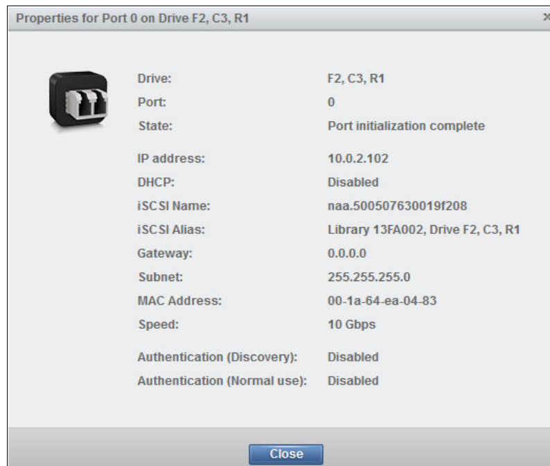
Figure 4-127 Ethernet port properties
