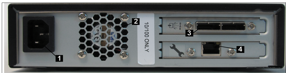
Figure 5-4 Rear view of the TS2280 tape drive
