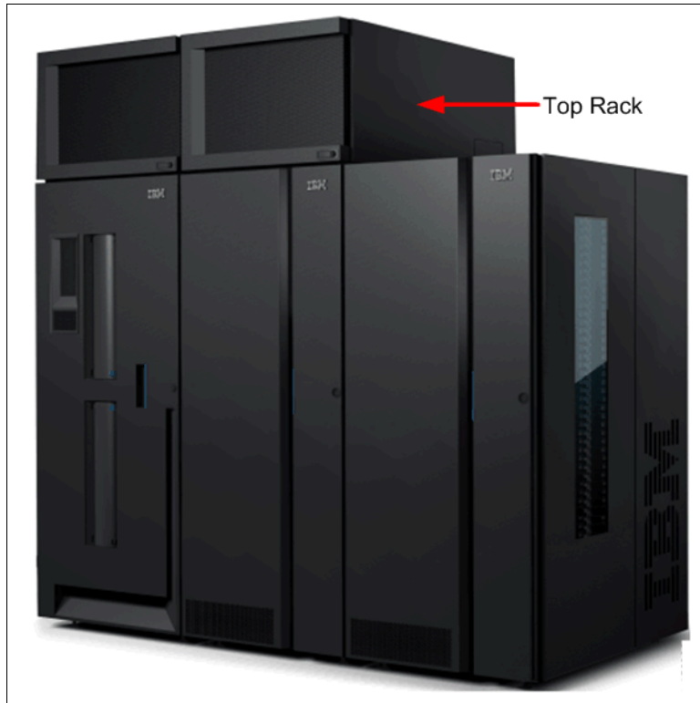
Figure 11-15 Tape library with top rack installed
