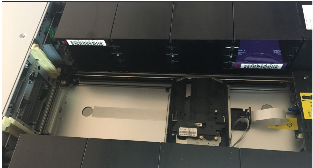
Figure 10-9 TS4300 tape library storage columns
