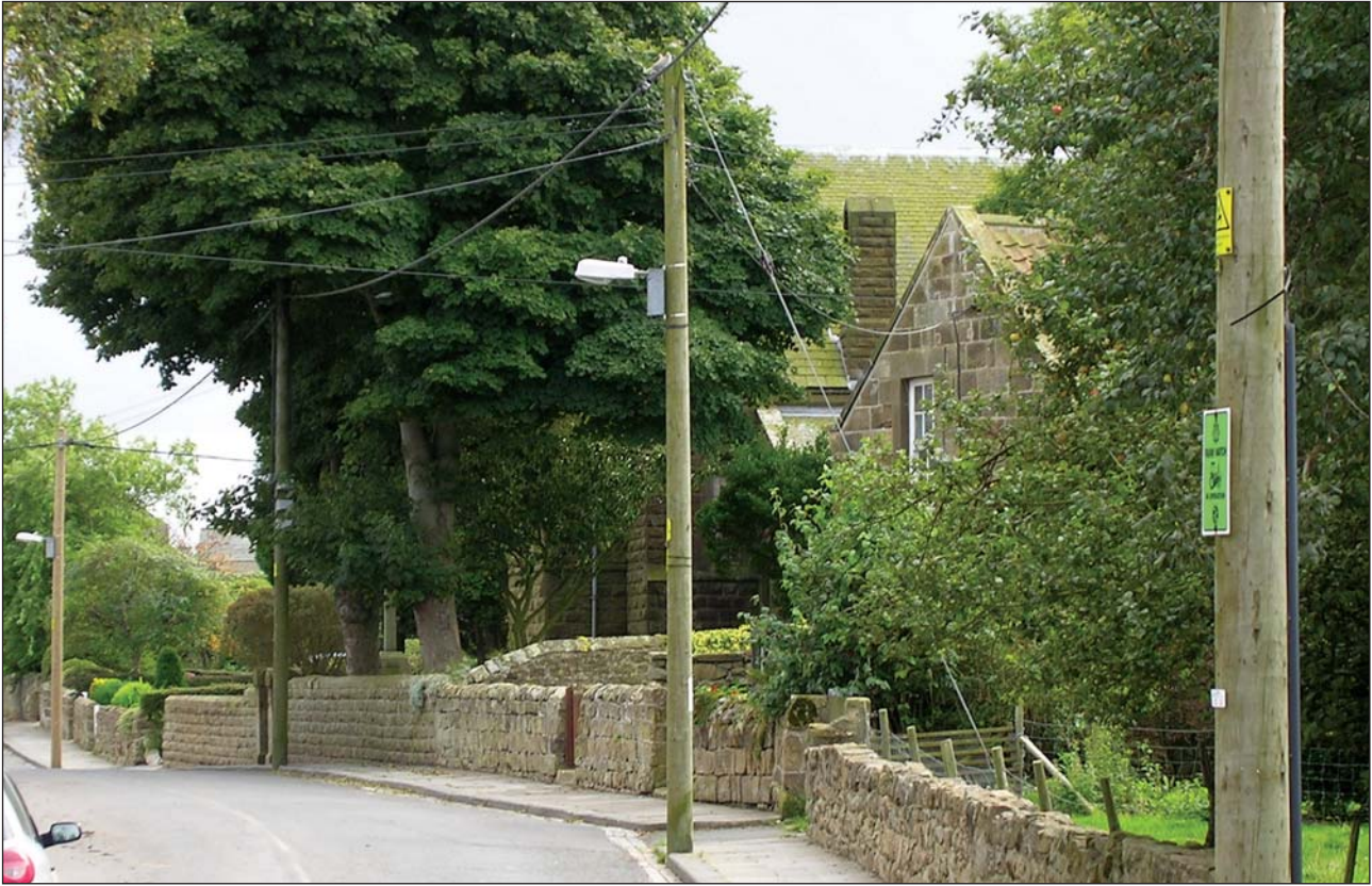
Picture 33. Timber poles used for overhead wires and street lighting
