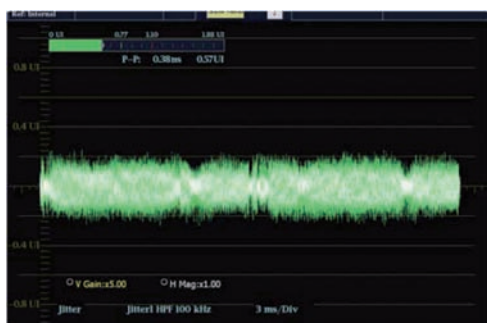
With the 100kHz filter applied the jitter readout shows 0.57UI of jitter.
