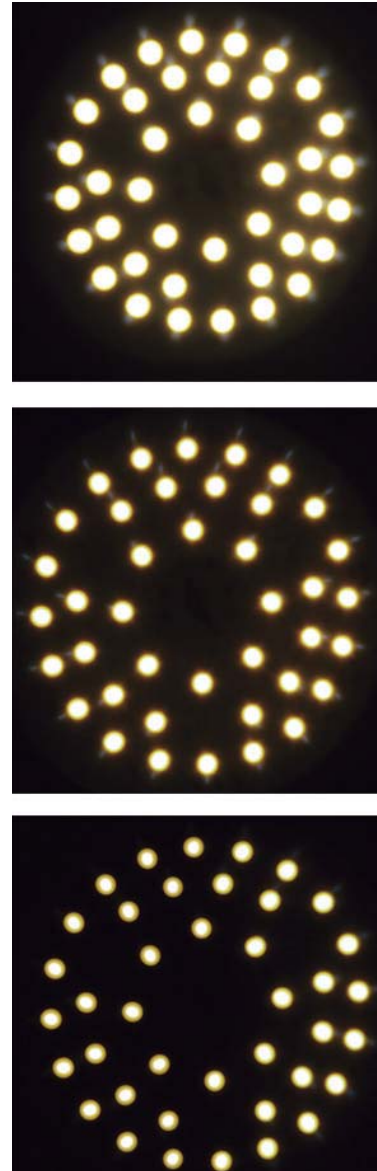
Figure 4. Even dimming with the EL01: an LED module with 5 W (top), 2 W (middle) and 1 W (bottom).
