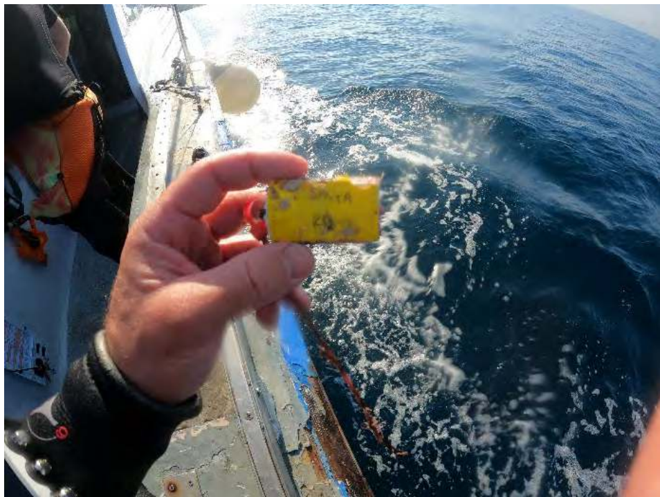
Figure 27: RCCA oceanographic sensors. Top: A deployed unit that collects data on pH, O 2 , and temperature of the water. Bottom: A recovered temperature logger (HOBO).
