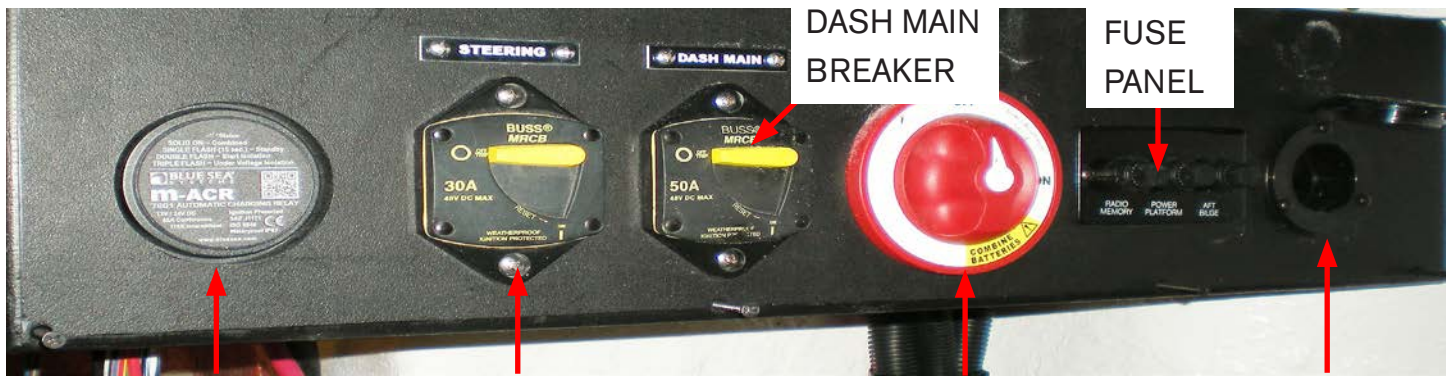
AUTOMATIC CHARGING RELAY POWER STEERING BREAKER
