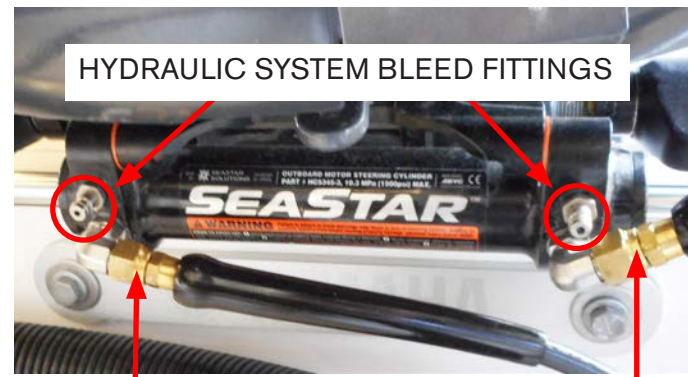
STEERING HARDWARE & HOSES AT ENGINE
