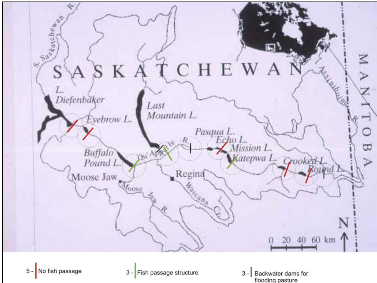
Figure 5. Qu'Appelle River basin and Qu'Appelle Lakes with existing dams and fish passageways identified.
