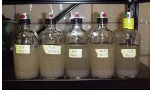
Sediment/Groundwater Microcosms from Ontario site - Produced lots of Ethene
