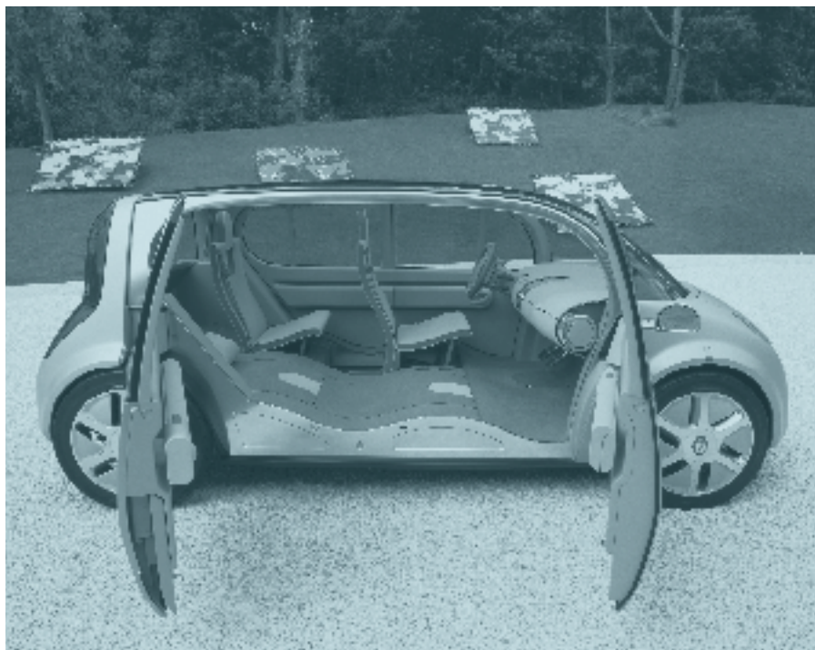
Press a button and Ellypse's "ingenious seats" recline into the floor, switching from "road" to "rest" position.
