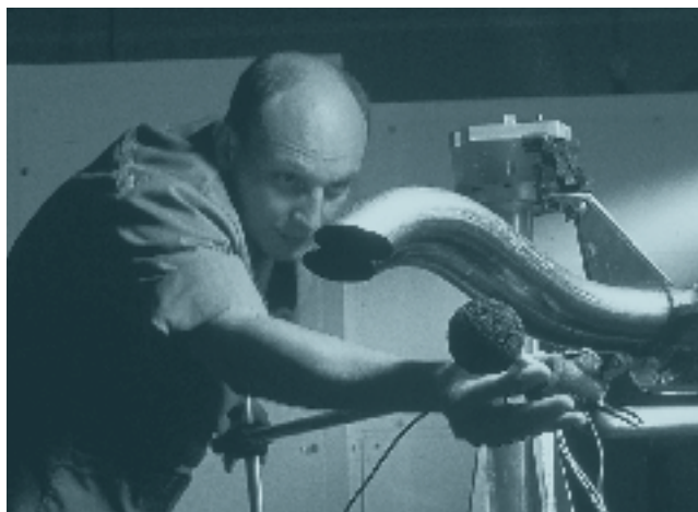
Acoustic testing to measure exhaust pipe noise.
