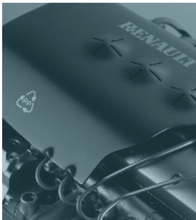
Ellypse's 1.2 16V dCi turbo engine develops 100hp with CO 2 emissions of just 85g per kilometer. Fuel consumption is 3.2 liters per 100 kilometers.
