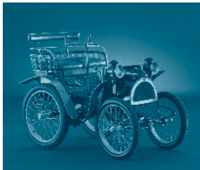
The starting-point for Renault was the Type A Voiturette, with its innovative direct-drive transmission.
