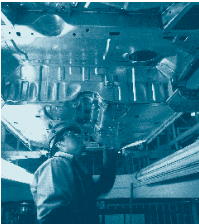
Controlling the quality of underbody welding on a Clio at Nissan Mexicana's Aguascalientes plant.
