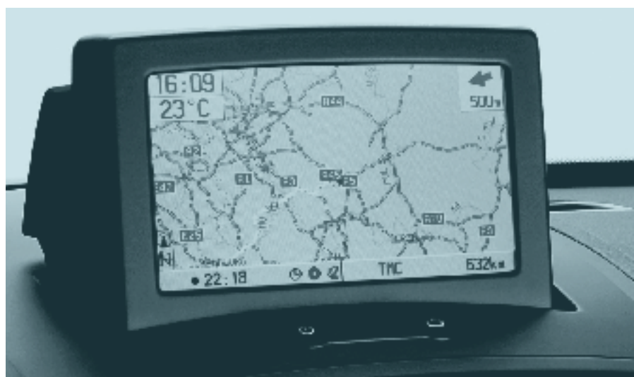
The tilt/fold wide-screen display of the Carminat Advanced Navigation system on Mégane II.
