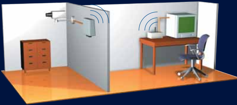
Standard camera plus universal wireless transmitter with indoor wireless multi receiver.
