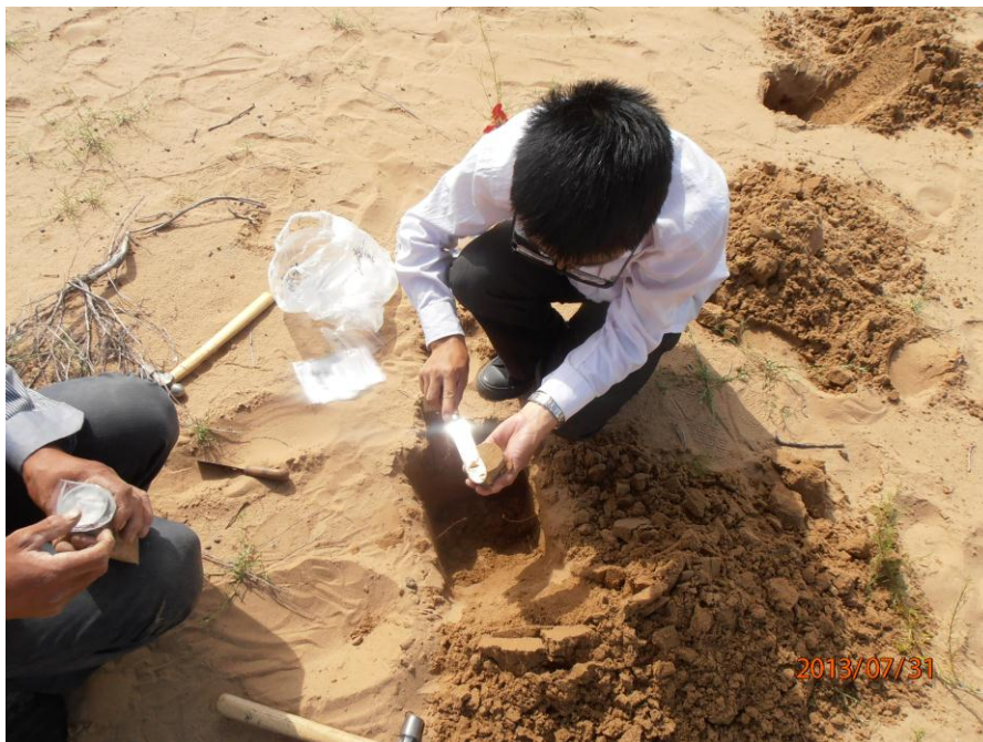
Fig. 22: Photo of taking soil samples for the analysis of soil bulk density with cutting ring method
