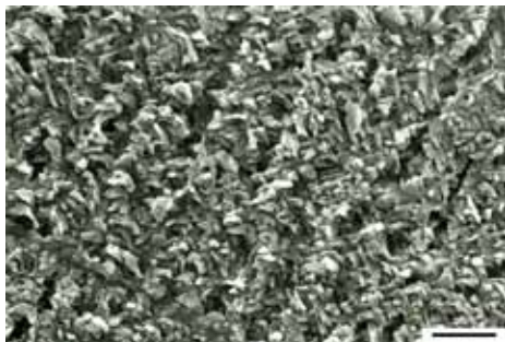
FIG. 76. Crossed acicular microstructure in the middle shell layer of arcticid Arctica islandica (LINNAEUS, 1767 in 1766–1768); polished and then acid-etched radial section; scale bar = 5 \mu\text{m} (Carter, new).
