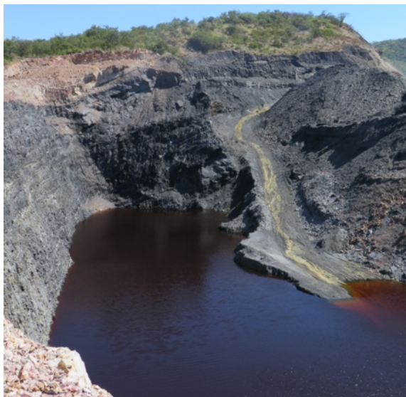
Suppl.-Figure 42 Pit lake at mining concession close to Sikabala effluent channel showing deep red colored water with high metal concentrations and pH around 2.6 at EFFSAN04 at 18°19'11.73"S, 26°28'16.32"E. Picture taken on 07.05.2019
