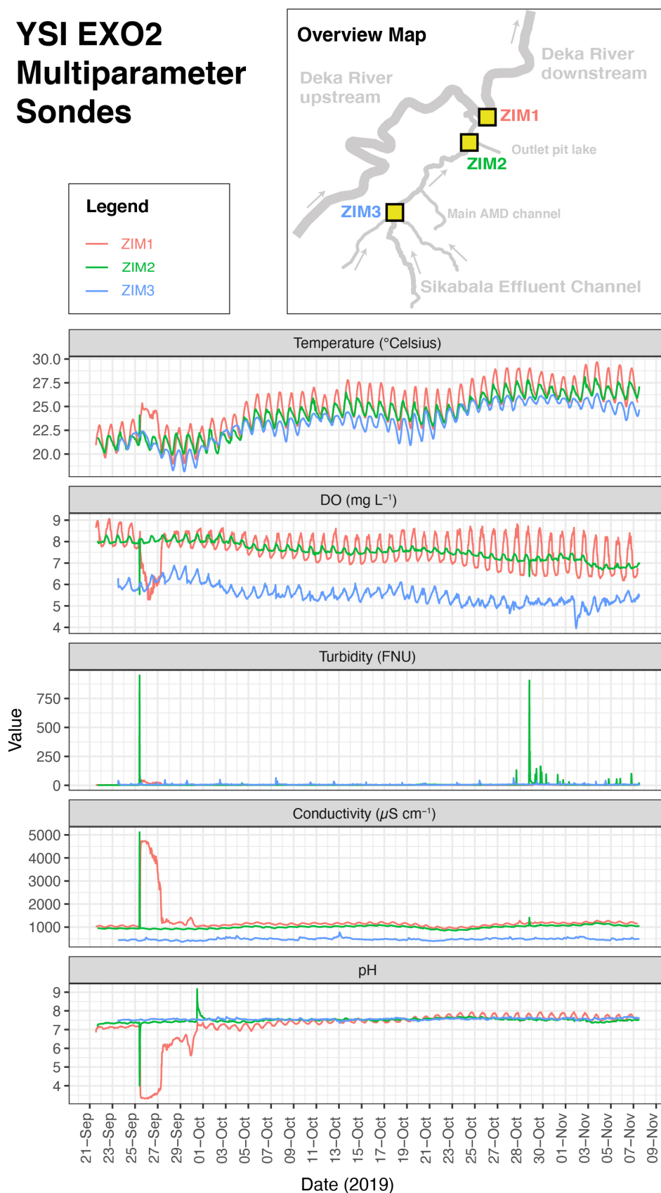
Figure 12 Temperature, dissolved oxygen (DO), turbidity, conductivity and pH measured by the YSI EXO2 Multiparameter Sondes (ZIM1, ZIM2, and ZIM3) from 23 September to 8 November 2019. Overview map shows probe locations: ZIM1 monitored the Deka River downstream of the Sikabala inlet. ZIM3 was located in Sikabala upstream of the main inflow of mine water and ZIM2 downstream of it.
