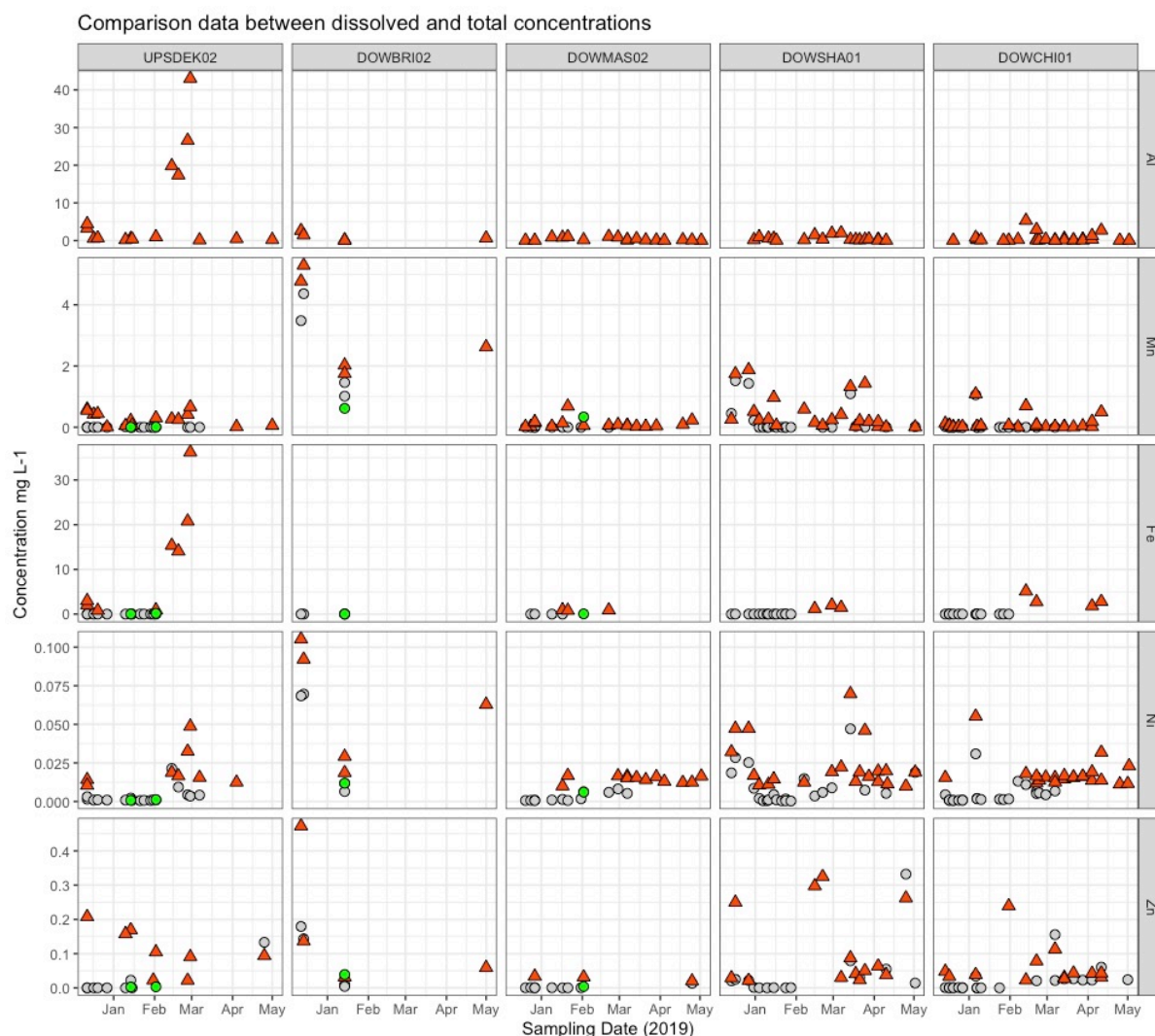
Suppl.-Figure 9 The same 112 grab samples from Deka River were analyzed for their dissolved (grey circles) and total concentration (red triangles). For 4 samples, a filtered and acidified sample was plotted for comparison (green circles)
