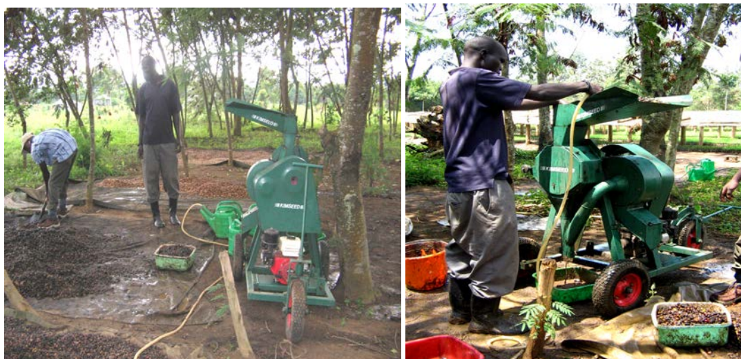
Seed collectors processing Measopsis eminii seed, using a Kim seed machine (Macerator) by Wet method of seed extraction.
