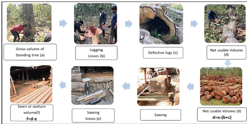
Fig 1: Overview of harvesting flow from standing tree to final outturn based on 16,17
