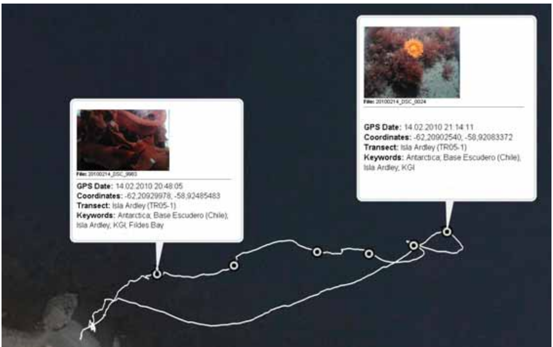
Geo-referencing of Underwater images using a diver-towed GPS buoy for positioning
