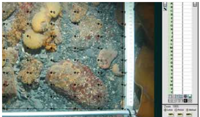
Determination of substrate coverage using the point count methodology of the software programme CPCe 3.6 [579]
