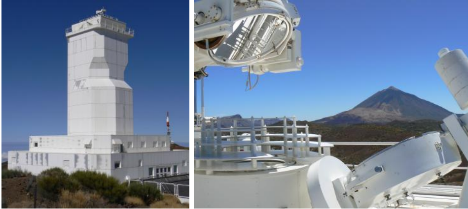
Figure 4.2.: The Vacuum Tower Telescope (VTT) at the Observatorio del Teide on Tenerife. On top of the tower (left panel) the dual mirror coelostat system (right panel) guides the light into the telescope.
