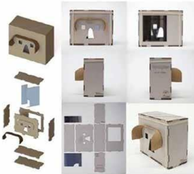
Figure 10. Cardboard Synopter - designed by Maarten Wijntjes (2016)
