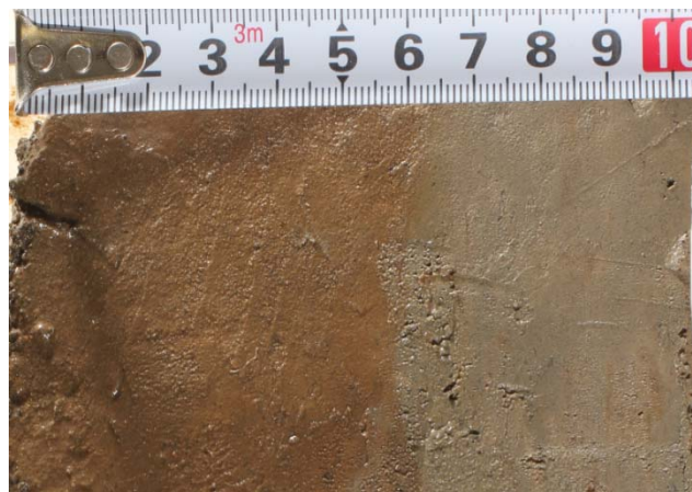
Fig. 23: Core SO250-4 (area A8) (©A. Mayorova). Description: 0-5.5 cm - Silty clay, brown, oxidized, soft consistence. On surface (0-1 cm) single rounded and sharp-edged pebbles (size about 1 cm).
