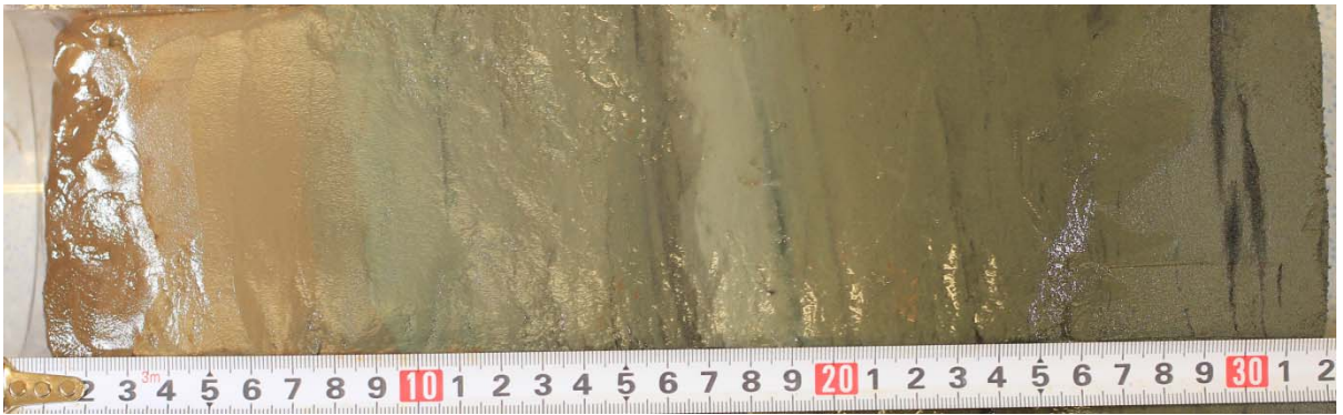
Fig. 30: Core SO250-79 (area A7) (© A. Mayorova). Description: 0-1 cm - Clay, brown oxidized, semiliquid. 1-3 cm - Clay, brown, soft, homogenous. 3-7.5 cm - Clay, grayish-brown, dense, stiff, viscous, at 4-5 cm - black lenses of silt with sharp border. 7.5-16 cm - Clay, grayish-olive, very dense, stiff, at 10 cm and 15.5 cm horizontally oriented rare black streaks of silt. 16-19 cm - Clay, lightly olive, very dense. A border between the layers is waterworn. At 19 cm - streak of dark green clay, very dense, stiff. 19-32 cm - Clay, olive, very dense, with horizontally oriented rare black streaks of silt.
