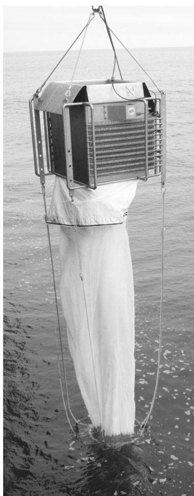
Figure 3: The Multiple-Plankton-Sampler (MPS Maxi combi; Hydrobios GmbH, Kiel, Germany) is made of stainless steel. The dimensions are 1.2 m x 1.2 m x 1.3 m with a weight of 420 kg. The gear shows a quadrate mouth opening of 71 cm width and high resulting in 0.5 m 2 effective net opening. The Multiple-Plankton-Sampler was used with five plankton nets of three times 335 µm and two times 100 µm mesh size. When deployed to maximum depth the net interval was 5,900 to 3,000 m (100 µm), 3,000 to 1,000 m (100 µm), 1,000 to 500 m (335 µm), 500 to 250 m (335 µm), 250 to 0 m (335µm). The gear is additionally equipped with CTD sensors (sea & sun) and an oxygen sensor (sea & sun).
