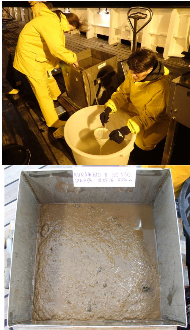
Fig. 54: Sieving of the overlaying water (upper) and the upper layer of bottom sediment collected by the box corer (lower).
