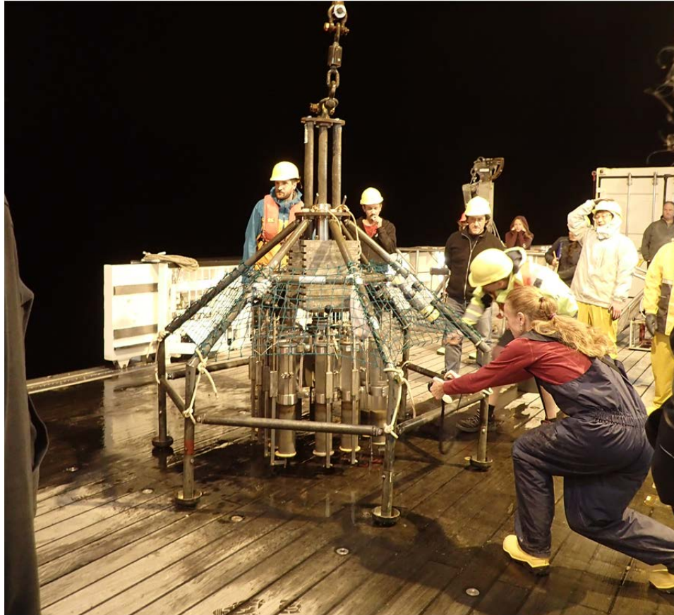
Figure 20: The multicorer after sampling the station 104 at 9540 m depth. Photo taken by: Hiroaki Fukumori.
