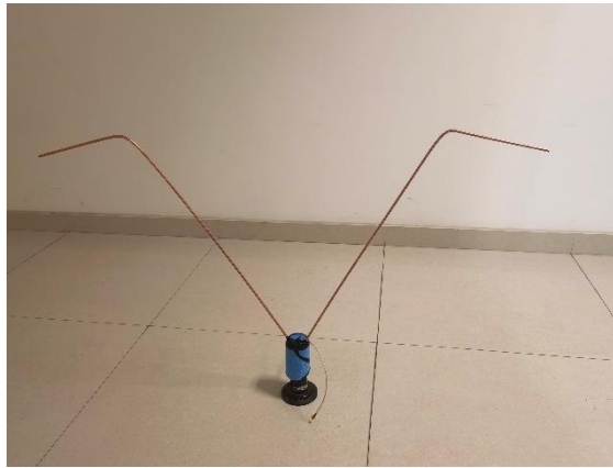
Figure 9: Homemade compressed V-shape dipole antenna
