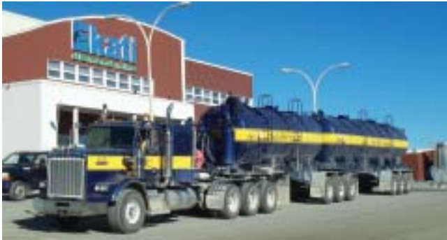
► Kete Whii tractor trailer unit with water tankers for dust suppression on roads in front of main facility entrance
