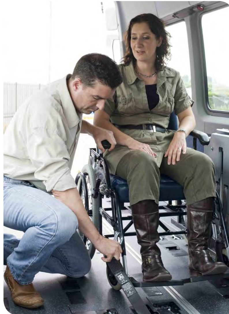
Flex-i-Trans enables a nine-seat minibus to be converted into a bus that can accommodate wheelchairs.
