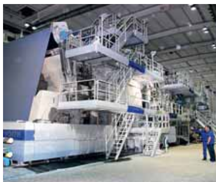
Test running of the new newsprint machine in Madrid began as planned at the end of the year. The machine will raise the mill's annual capacity by 300,000 tonnes.
