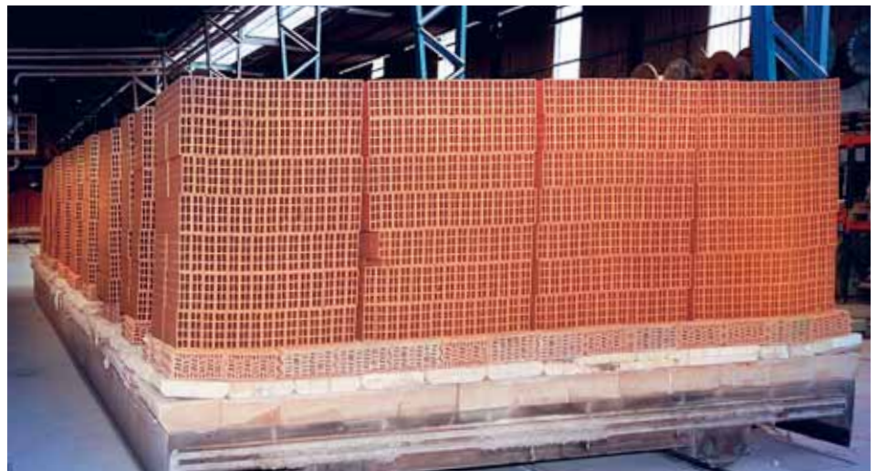
The sludge produced at the Madrid mill from the de-inking of recovered paper is used as fuel and as a binding agent in factories that manufacture building blocks.
