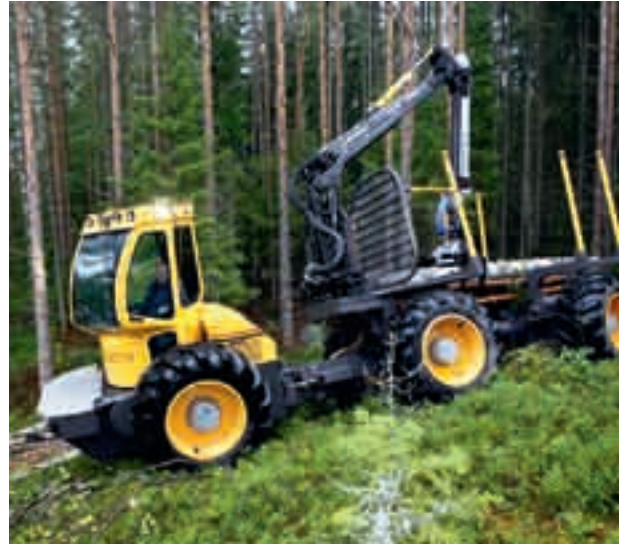
The El-Forest hybrid electric harvester consumes 30–50 per cent less diesel fuel than a conventional harvester. The harvester in the photo is a prototype. Holmen will take delivery of its first El-Forest in 2010.
