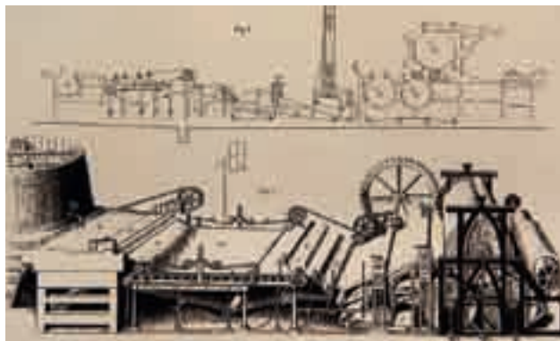
Holmen installed one of Sweden's first paper machines in 1837. It created a sensation with its continuous production of paper in long webs.
