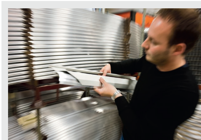
The special profile that joins the roof and walls of Kabe camper vans and caravans is the result of a long, complicated process.
