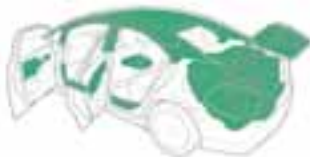
Promoting use of Ecological Plastic for plastic parts (Photo: Parts of the SAI where Ecological plastic is used)
