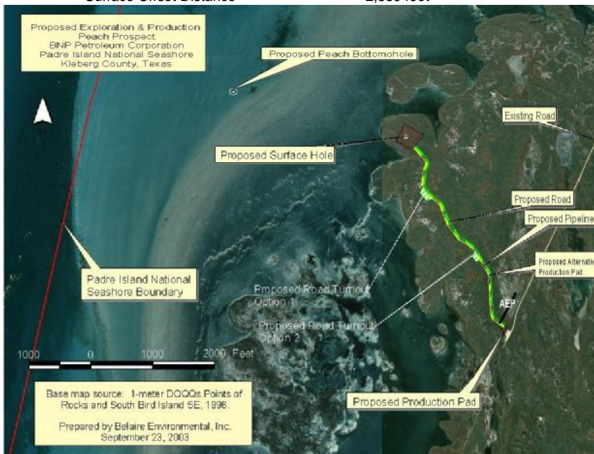
Figure 3. Surface and bottom hole locations for the Dunn-Peach # 1 Well.
